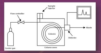
I write and help execute instructions for building and testing of the Gas Chromatograph subsystem. These build procedures include leak and proof testing of pressurized and vacuum components. It also involves performing functionality tests and safe to mate measurements of valves, platinum resistance thermometers, heaters, regulators and pumps.
