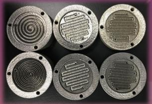
I designed several 3D printed and machined prototypes for the reactor that is used to oxidize water. This involved collaboration with manufacturing engineers to create different geometries and substrates. These caps were then treated using various methods to create a photocatalytic layer.
