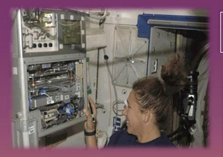
miniTOCA is a NASA JSC and JPL oxidation and sensor instrument intended to replace the carbon analysis system currently monitoring the water on the ISS.
